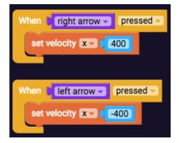
Duplicate both of these blocks and click on "pressed" to change it to "released". Set the x velocity to "O" in both blocks.
